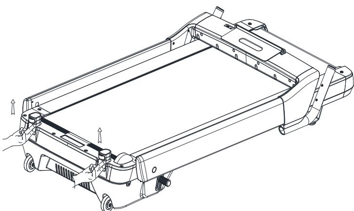
4.Before moving the treadmill, pull out the supporting moving wheels according to the drawing, to ensure the standing stability of the bracket.
