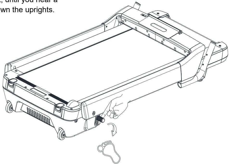
3.Fold the pad bracket. Pull the pad bracket to the right according to the drawing. Then finish by turning down. Need to take off the handrails when you fold the product.
